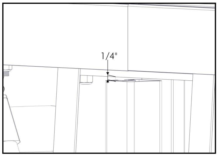
WITH THE CANOPY FRAME AND TILT KIT INSTALLED, SWING THE LOWER ACTUATOR MOUNT AND ACTUATOR TOWARDS EXTENSION TUBE (FIGURE 2.3). SLIDE THE EXTENSION TUBE UP OR DOWN TO CENTER THE LOWER ACTUATOR MOUNT BRACKET ON THE EXTENSION TUBE. TORQUE 60 FT-LB (FIGURE 2.4).
