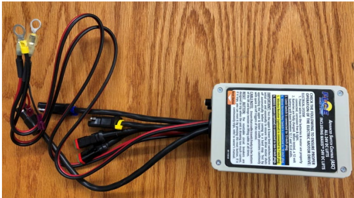
FULL 24V ASC HARNESS (INCLUDED IN VSD DRIVE KIT)
