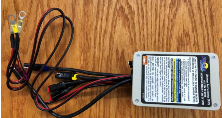
FULL 24V ASC HARNESS (INCLUDED IN VSD DRIVE KIT)
