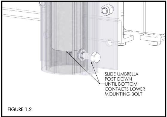
THEN, INSTALL A 3/8" X 1-3/4" BOLT INTO THE MOUNTING HOLE AND INTO THE RIVET NUT ON THE TABLE POST (FIGURE 1.3). TIGHTEN UNTIL THERE IS NO EXCESS MOVEMENT IN THE UMBRELLA POST. DO NOT OVERTIGHTEN, AS YOU CAN CRUSH THE UMBRELLA POST (FIGURE 1.4).
