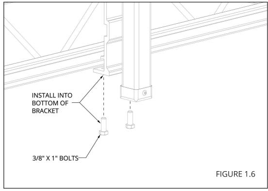
TORQUE BOLTS TO 6 FT-LB MAXIMUM (FIGURE 1.7). REFER TO WATER ACCESSORY RACK INSTRUCTIONS TO COMPLETE INSTALLATION.
