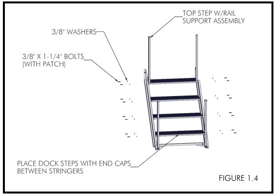
FOR 8 STEP STAIRS, A MID STEP HANDRAIL SUPPORT ASSEMBLY IS PLACED ON THE FIFTH SET OF HOLES FROM THE BOTTOM OF THE STAIRS (FIGURE 1.4A). SNUG DOWN ALL FASTENERS, BUT DO NOT OVERTIGHTEN. OVERTIGHTENING WILL PREVENT STEPS FROM LEVELING THEMSELVES (FIGURE 1.5).
