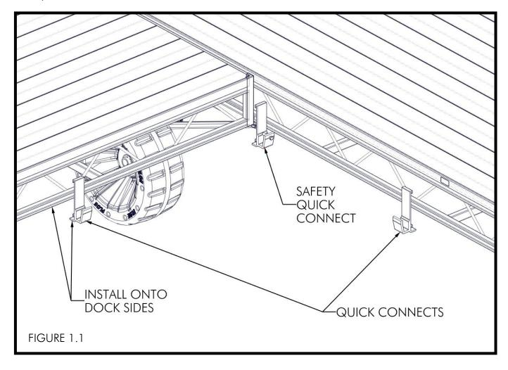
POSITION THE CONNECTS ON THE DOCKS WITH THE SPECIFIED DIMENSIONS SHOWN FOR EACH SIZE WEDGE. ALL MEASUREMENTS ARE MADE FROM THE CORNER OF THE SUNDECK/OFFSET DOCK (FIGURE 1.2 & 1.2A). THE FOLLOWING DIMENSIONS ARE SUGGESTIONS AND MAY CHANGE DUE TO THE INDIVIDUAL'S DOCK LAYOUT. AS A GENERAL RULE, PLACE THE QUICK CONNECTS AS FAR OUT AS POSSIBLE.
