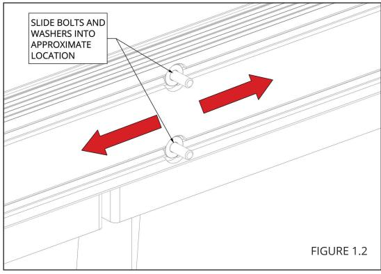
POSITION THE HAND RAIL ON THE DOCK SIDE SO THAT THERE IS AN EQUAL DISTANCE ON BOTH ENDS OF THE DOCK BETWEEN THE END OF THE DOCK TO THE BRACKET (FIGURE 1.3). PLACE THE HAND RAIL ONTO THE BOLTS BY ALIGNING THE HOLES ON THE MOUNTING BRACKETS (FIGURE 1.4).
