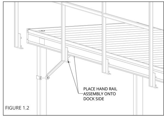
ATTACH THE HAND RAIL TO THE DOCK BY INSTALLING (2) 3/8" X 1" BOLTS INTO EACH BRACKET (FIGURE 1.3). TORQUE ALL BOLTS TO 6 FT-LB MAXIMUM (FIGURE 1.4).
