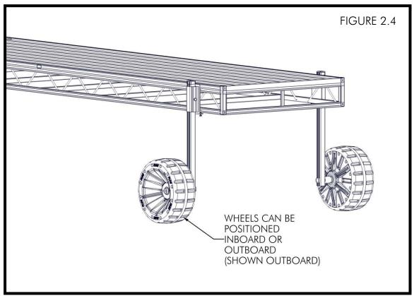
ADJUST THE WHEEL KITS TO ACHIEVE THE DESIRED HEIGHT AND DOCK LEVELNESS. ONCE SET, TORQUE THE 1/2" BOLT TO 50 FT-LB. SLIDE A VINYL CAP ONTO THE END OF EACH TUBE (FIGURE 2.5).
