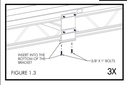
TORQUE BOLTS TO <u>6 FT-LB MAXIMUM</u> (FIGURE 1.4). PLACE THE FURNITURE POCKETS (**SOLD SEPARATELY**) ONTO THE BRACKETS AND ATTACH THEM WITH (4) 3/8" NYLOCK NUTS PER BRACKET (FIGURE 1.5). TORQUE NUTS TO 35 FT-LB (FIGURE 1.6).
