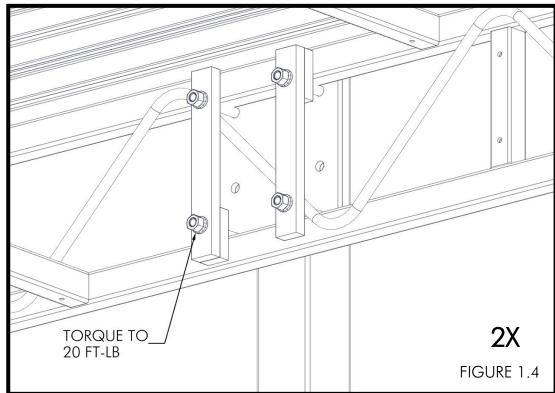
PARK BOAT ON LIFT AND SET THE POSITION OF BOW STOP UPRIGHTS BY SLIDING THE UPRIGHTS UNTIL THEY CONTACT THE BOAT. THE PVC UPRIGHTS SHOULD NOT BE BENT FORWARD OR TOWARDS THE SIDES OF THE HULL AND THE TOP OF THE TUBE SHOULD BE 6-8 INCHES ABOVE THE RUB RAIL WHEN THE BOAT IS FLOATING INSIDE OF THE LIFT. TORQUE 1/2" NYLOCK NUTS TO 20 FT-LBS (FIGURES 1.5 & 1.6).
