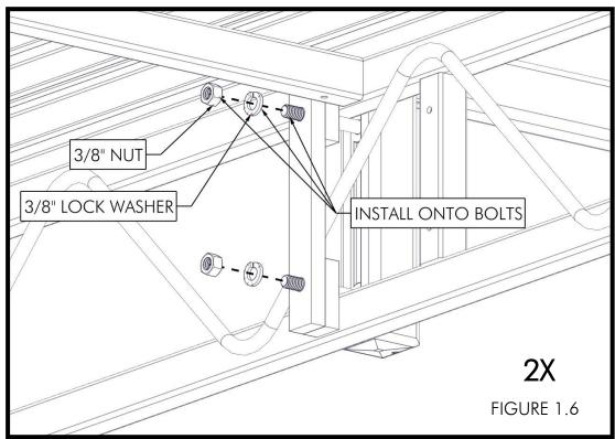
WHILE ENSURING THE UPRIGHTS ARE SQUARE TO THE TOP OF THE DOCK, TORQUE NUTS TO 20 FT-LB (FIGURE 1.7).
