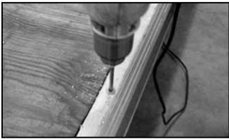
1. Drill the five (5) rivets out of the top of the rear bumper.
