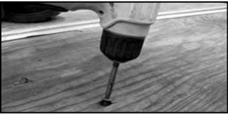
**3.** Drill the rivets or remove screws out of the plywood and slide the plywood out the back of the trailer.
