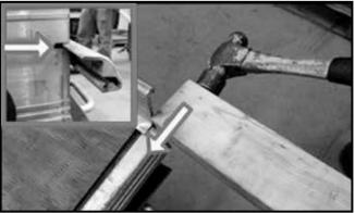
**2.** Using the block of wood, drive the rear bumper out the slotted side panel.
