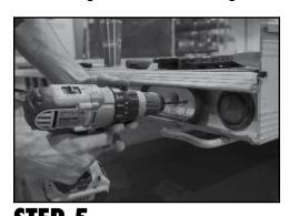
1) Drill out the rivets from the plate, and pull the
