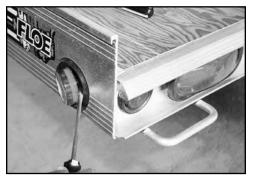
Inserting the lights too far into rubber grommet will cause the back of the it to bulge allowing moisture in. Check the back of the grommet and make sure it is not bulging.
