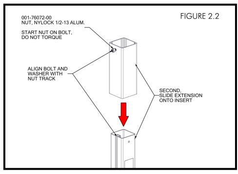
FIRST, SET HEIGHT OF EXTENSION TUBE 7-3/8" FROM TOP OF CORNER POST. THEN, SWING LOWER ACTUATOR MOUNT AND ACTUATOR TOWARDS EXTENSION TUBE (FIGURE 2.3). EXTENSION TUBE WILL BE APPROXIMATELY 5-3/16" FROM TOP OF TUBE TO TOP OF ACTUATOR MOUNT. TORQUE 60 FT-LBS (FIGURE 2.4).
