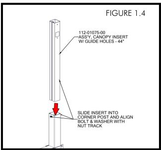
THE MAXIMUM HEIGHT OF THE INSERTS IS 38" (6" OF ENGAGEMENT IN THE CORNER POSTS). THE MINIMUM HEIGHT OF THE INSERTS IS 26" (18" OF ENGAGEMENT IN THE CORNER POSTS) (FIGURE 1.5). TORQUE ½" NUT TO 60 FT-LBS (FIGURE 1.6). PROCEED TO INSTALL MAXIS CANOPY BY REFERRING TO MAXIS CANOPY FRAME INSTRUCTIONS.
