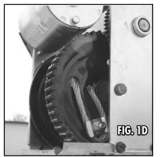
Attach the new cable to the drum as shown in FIG. 1D and torque to 5 ft/lbs.
