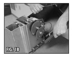
Pull open and remove plastic winch cover. NOTE: It will be difficult to get the cover around the gears (FIG. 1B).
