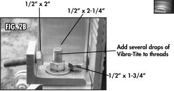
IMPORTANT NOTE: Vibra-Tite takes 24 hours to fully cure. Do not operate the winch until the appropriate amount of time has elapsed while maintaining the 12:00 o'clock and 6:00 o'clock eye nut position.
