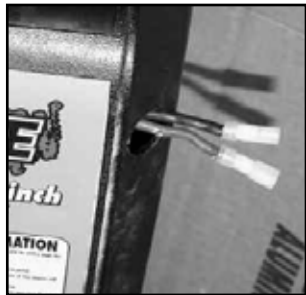
Fig. 8A Push wires out hole in cover
