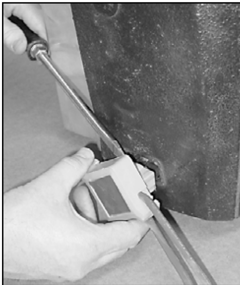
Fig. 1 Removal of Rotary Switch
