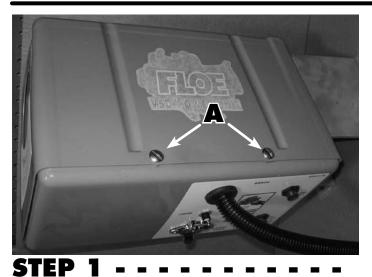
Remove the four screws in the cover, two on each side see (A). Remove the old base and unplug it from the motor see (B). Unplug clip by lightly pushing the top part of the spring clip and pulling clip apart see (C).
