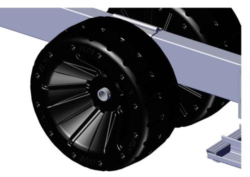
PLACE WASHER ONTO SPINDLE. PLACE SPINDLE CLIP INTO ONE OF THE DESIGNATED HOLES AND SLIDE OVER UNTIL IT SNAPS INTO THE OTHER HOLE.
