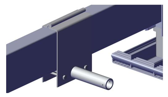
PLACE 3/8-16 NUTS ON BOLTS. TORQUE TO 5 FT-LBS.
