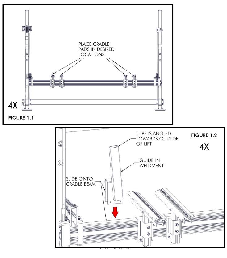
ATTACH WELDMENTS TO THE CRADLE BEAM USING (2) 3/8" X 4" BOLTS AND (2) 3/8" NUTS. **DO NOT TORQUE AT THIS TIME** (FIGURE 1.3). SLIDE PVC PIPES ONTO THE TUBES ON THE GUIDE-IN WELDMENTS (FIGURE 1.4).
