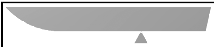
Illustration A: above shows the boat's balance point of center of gravity (CG).
