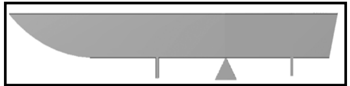
Illustration B: shows the boat's center of gravity (CG) centered between the two main lift beams – each of the lift beams is supporting the same amount of weight.
