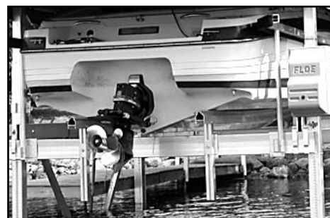
Fig. 39 - Less desirable bunk placement - Ideally in the above example, the lift bunks would have been positioned wider as in Figs. 37-38 . Doing so would have allowed the bunks to be set higher, preventing the vertical tubes from sticking so far below the main lift beam.
