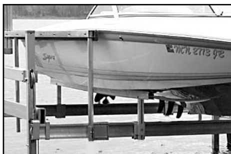
Fig. 38 - Bunk height recommended for inboards - The bunks are spread wide and the hull is lifted so that the running gear on an inboard can pass over the main lift beam without making contact.
