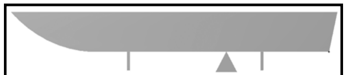
Illustration C: shows a boat's center of gravity (CG) improperly positioned so that it extremely overloads one of the main lifting beams.
