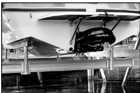
Fig. 37 - Ideal bunk placement - Note that the bunks are spread out to the widest position on the boat hull. They sit nicely into the contour of the hull and the keel has plenty of clearance above the main lift beam. If possible, this is the most ideal bunk placement for non-inboards.
