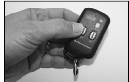
Fig. 66: Wireless remote is an optional feature. The wireless remote control will operate both the lift and the lighting system.
