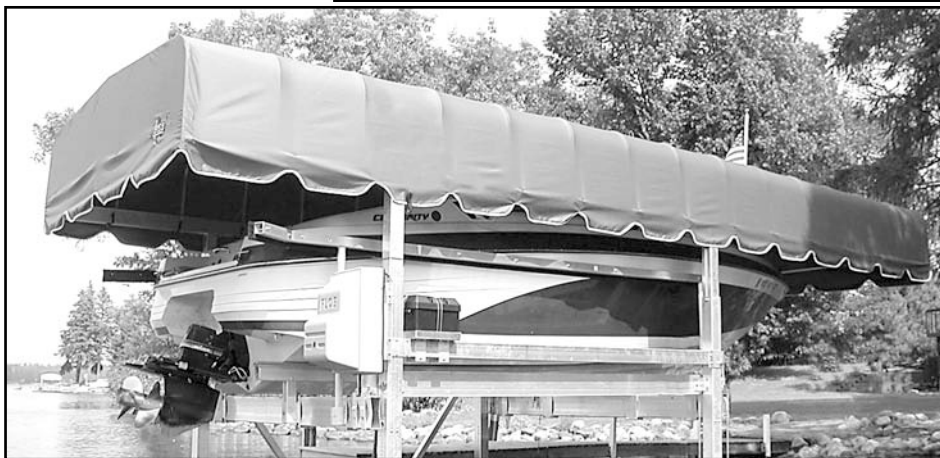
Fig. 45 - Boat shown in proper position so that as much weight as possible is transferred to the front beam. The canopy is positioned so that it covers the entire boat.
