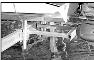
Fig. 44 - A motor stop can help achieve correct location every time and prevent your motor from hitting the rear main cradle lift beam.
