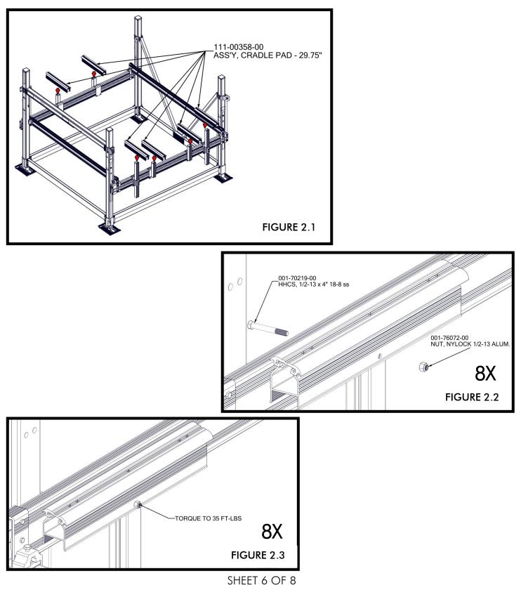
POSITION THE (4) CENTER CRADLE PAD ASSEMBLIES, (2) PER CRADLE BEAM, AND (2) OUTER CRADLE PAD ASSEMBLIES BASED ON THE WIDTH OF THE BOAT. PADS MUST BE POSITIONED SO THAT THEY UTILIZE THE CHINE OF THE HULL, AS THIS WILL HELP TO KEEP THE CRADLE PAD ASSEMBLIES VERTICAL (FIGURE 2.4 & 2.4A).
