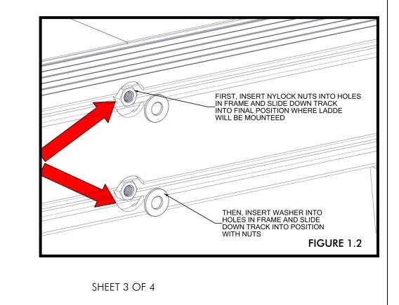
ATTACH LADDER TO DOCK SIDE USING (4) 3/8" X 2-3/4" BOLTS. SLIDE THROUGH THE UPPERMOST HOLES IN THE LADDER AND INTO THE WASHERS AND NYLOCK NUTS (FIGURE 1.3). ADJUST LADDER POSITION IF NECESSARY, THEN TORQUE TO 30 FT-LBS (FIGURE 1.4).
