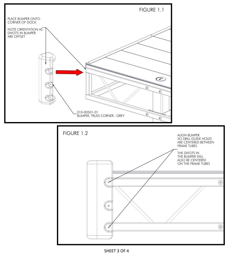
WHILE HOLDING THE BUMPER SECURELY TO THE CORNER OF THE DOCK, DRILL (4) HOLES THROUGH THE BUMPER AND INTO THE DOCK FRAME TUBES USING A #9 DRILL BIT (FIGURE 1.3). INSTALL (4) 3/16" X 1/2" RIVETS INTO THE BUMPER USING A RIVET TOOL (FIGURE 1.4).
