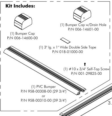
4. Slide the bumper caps over the bumper extrusion. Top cap: Pull the edge of the cap out and over the tape. Pull the cap all the way on and make sure it adheres to the tape. Bottom cap: The cap with the drain hole should be installed on the bottom end of the bumper with screw 1/2" up from edge and centered.
