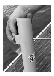
**3.** Place tabs on screws. Do not tighten.
